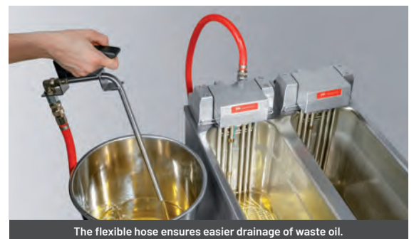
The flexible hose ensures easier drainage of waste oil.
